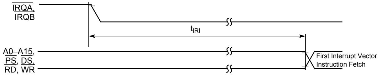
Figure 3-17 Interrupt from Wait State Timing
