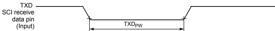
Figure 3-28 TXD Pulse Width
